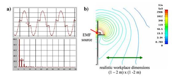
Fig. 1 Examples of selected parameters of EMF: (a) spectrum of frequency components of magnetic fields produced by tyristors supplying system [fundamental frequency of 50 Hz and harmonics] and (b) spatial distribution in front of dielectric heater
