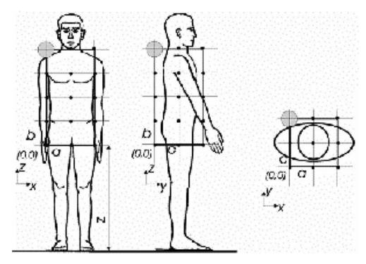
Fig. 2 The grid of spot measurement's locations fixed by product standard EN 50357 for the procedure of assessment of EMF emission form electrical appliances—measurements in 45 locations covering the  $0.3 \times 0.3$  m cross section of the torso of exposed person location
