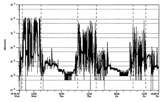
Fig. 1. Three days of measurement for a metal worker reporting: First day, 5 h of MMA welding; second day, 5 h of MIG/MAG welding; last day, 3 h of MIG/MAG welding. The vertical dashed lines indicate the beginning and finishing of work periods. The record comes from a "standard" exposure meter ( $0.01-70 \ \mu\text{T}$  in three axis) and some overloading of the instrument is found in the first day of measurement.
