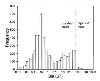
Fig. 3. Histogram of magnetic field values in the three work periods of the measurement presented in Figures 1 and 2. Values below 63  $\mu$ T in Figure 1 and values above 63  $\mu$ T in Figure 2 are combined. Number of measurement values 7844 (21.5 h). Arithmetic mean 9.73  $\mu$ T.
