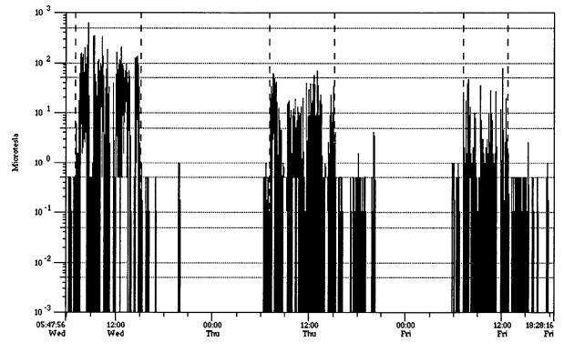
Fig. 2. Three days of measurement with a "high field" exposure meter (range,  $1-7000 \,\mu$ T) same worker and measurement period as in Figure 1.
