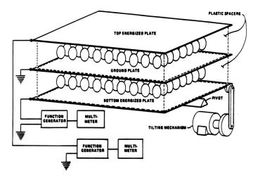
**Figure 4.** Diagram of the exposure system for the eggs during incubation. The top volume was energized with one frequency and the bottom volume was energized with the other frequency. This system was housed in a humidified walk-in incubator room maintained at  $36^{\circ}$ C.
